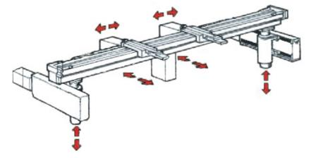
All backgauges are equipped with our precision machined fingers with multiple gauging points for longer part forming
