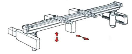
All backgauges are Low Profile with the fingers being the tallest component allowing easier material positioning
