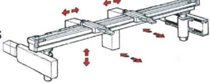
All backgauges are available for 100 to 1,000 ton press brakes in dual and triple drives in 24" or 48" travel
