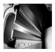
**Conventional Tooling**—Adjustable, conventional, four way, single V plus all other die requirements available with model AB press brakes
